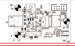
The USB Interface connects a PC with a Braille Line assembled with metec Braille Modules. For Flat20 Braille Line or B11,B12, P16 Braille Lines with separate 200V power supply
